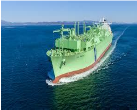
Figura 2 - FSRU - Floating, Storage and Regasing Unit (GNA, 2020).
